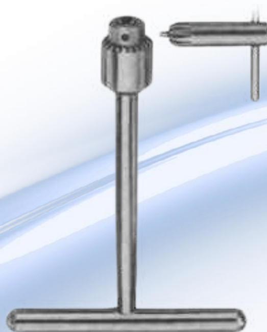
MES-23-155 Drilling chuck, cannulated for shanks up to 4.5 mm diam.. And for triangular shaft width across flats 4.7 mm
