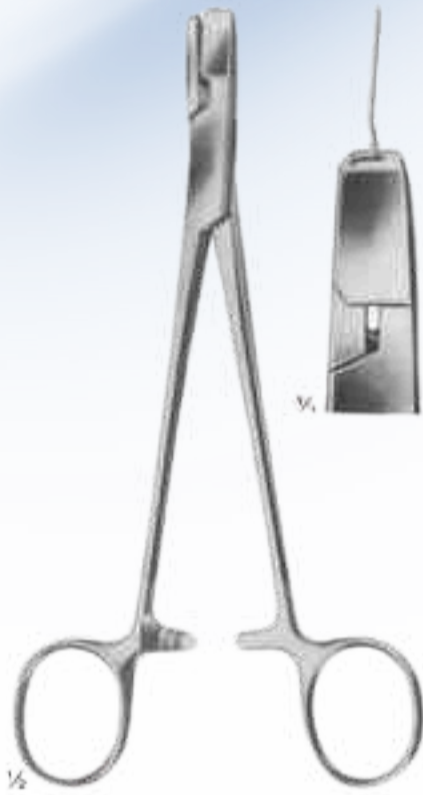
MES-23-167 DUROGRIP Holding forceps for cerclage wire, with lateral jaws to avoid wire slipping off 170 mm
